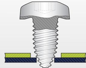
Forward extrusion with diametrically opposed thread engagement.
