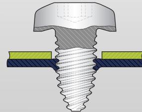
Increased core diameter approaching the underside of the head causes additional forward and backward extrusion providing increased thread engagement.
