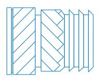
Offering high pull-out/torque performance. Hi-Tork is recommended for high fill plastics with reduced installation depth, is tolerant of molding process variables and provides high process capability.
