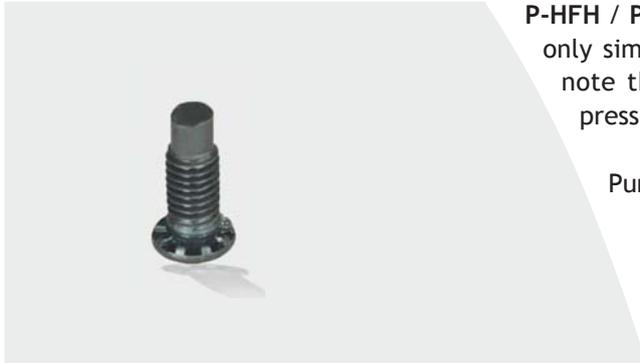
**P-HFH / P-HFHS SELF CLINCHING STUDS** are easy to install because only simple tooling is required. However, it is very important to note that they must always be installed by a squeeze action press rather than a hammer blow.
